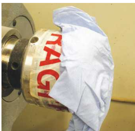
▲ Pic.31 Less friction drives the bowl between centres. Mount something on the headstock and use some rubber and tissue on the face so that you will not mark the centre of the bowl
